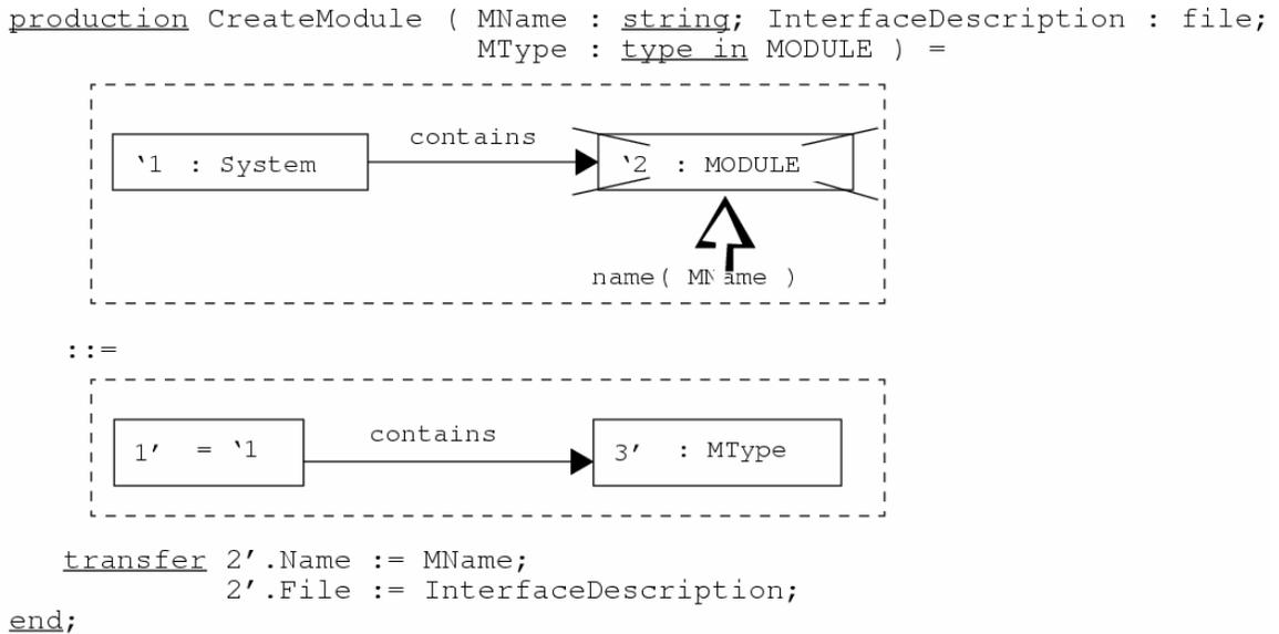
Figure 8. Example specification of a graph transformation [20]
