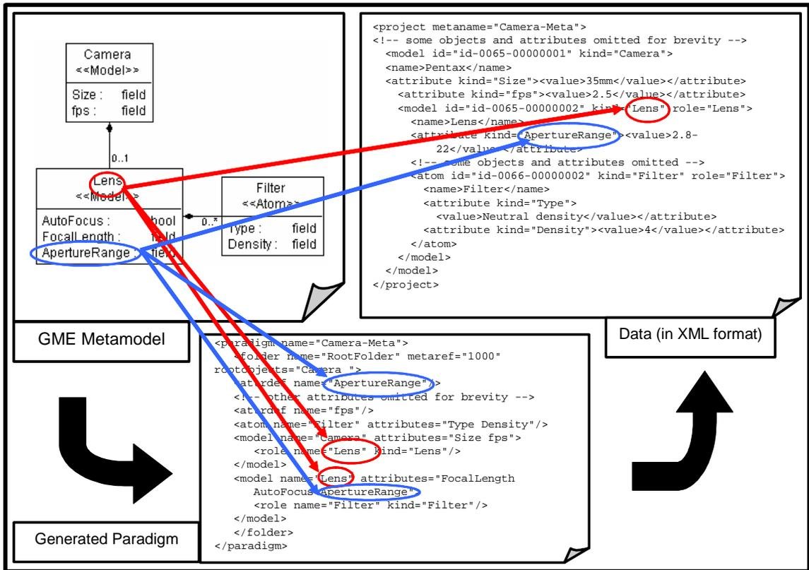
Figure 30. An example domain-specific modeling language created using the UML metamodeling environment. The red draws attention to object type and its dispersion throughout the paradigm and transform, while blue draws attention to the attribute type
